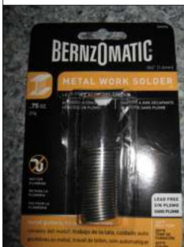
The 'metal work' solder – that does not adhere to brass at all.....lead-free it may be, but is also free-of-use for aeromodellers as well.....no indication on packaging that it has no affinity for brass.
