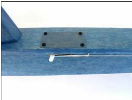
I installed the servo inside the fuselage and wound the DT line around a peg to reduce the load on the servo.
