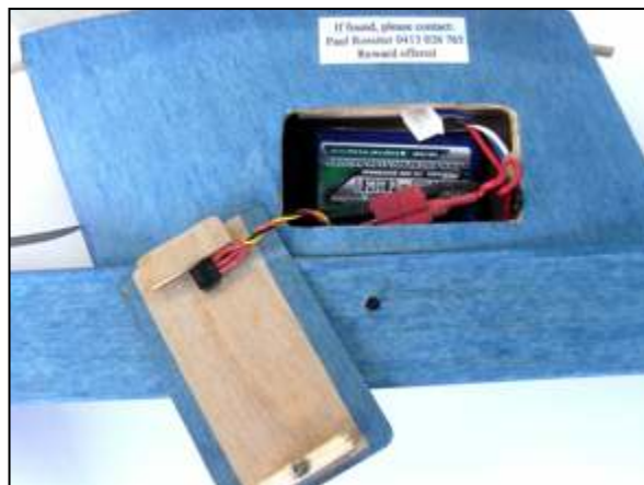
I mounted the battery in the pylon
