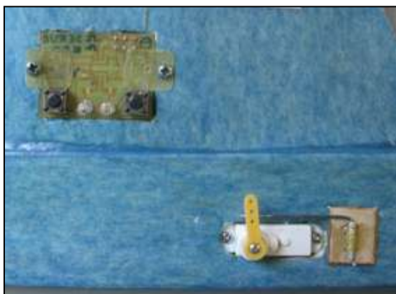
I installed the servo inside the fuselage and wound the DT line around a peg to reduce the load on the servo.
