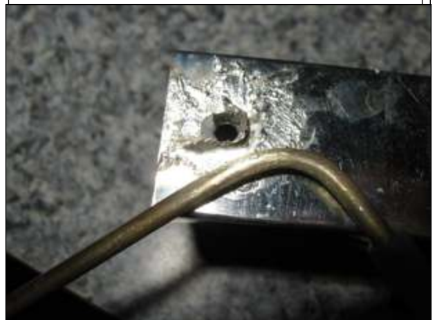
The tank and brass tube – solder adheres to tin alright, but not the brass tube.....Quite a puzzle trying to get the tube soldered in – until it was noticed the brass simply did not adhere, no matter how clean and well prepared.
