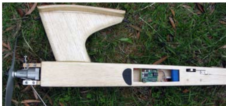
Dixie timer side. DT servo with release arm behind the timer hatch. The large cutout is a bit unplanned but it does make it easier to hold the servos in place while the screws are fitted. The blue foam rubber holds the 130mAh Lipo battery in place.
