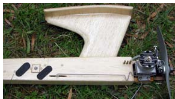
Dixie, motor side showing throttle servo arm, start button (between finger grips - skateboard grip tape is useful)
