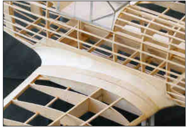
Wings halves plug into fairings, fixed to the body
