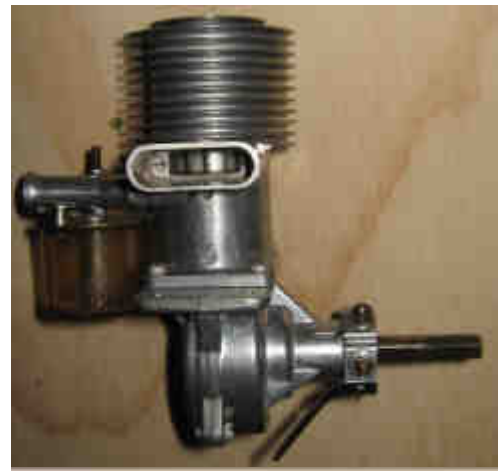
The Forster 99. The engine has a reputation of being very tractable, if not exactly a powerhouse. This one seems to have been little run, if at all, and should be a goer but needs a prop driver, needle valve and adaptor from whatever thread is in the head to 1/4-32.....one day.
