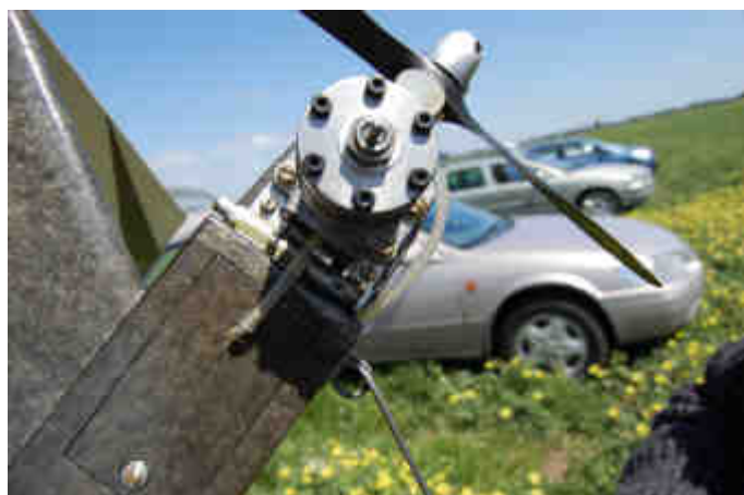
Peter Lloyd's reworked OS15 & showing a control line cut out made to suit Free Flight
