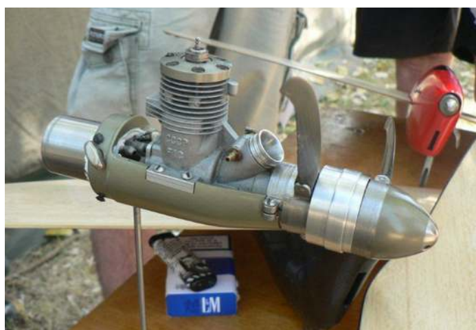
F1C motor with single folding contra rotating props, seen on a stand at the world control line champs. Did not ask the price I guess I should of just for interest.
