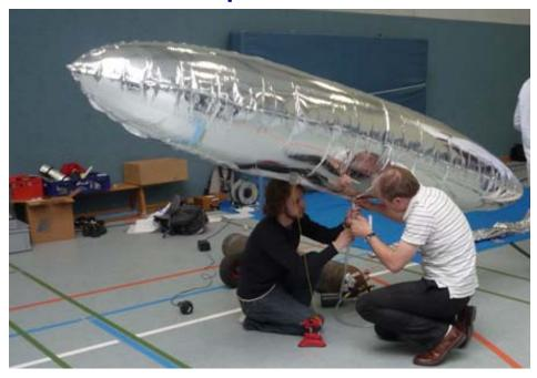
AEROSTATS are lighter than air models. We have two main types of aerostats: Hot air balloons and Airships. Airships obtain their sustentation from gas (or from hot air), have propulsion units and can be directed.
