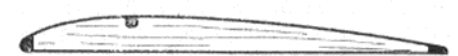
FIG. 15. NEARER BALANCED STRUCTURE. CENTRE OF SPANWISE BENDING RESISTANCE NEAR CENTRE OF COVERING TENSION BENDING -PREVENTS BOW.
